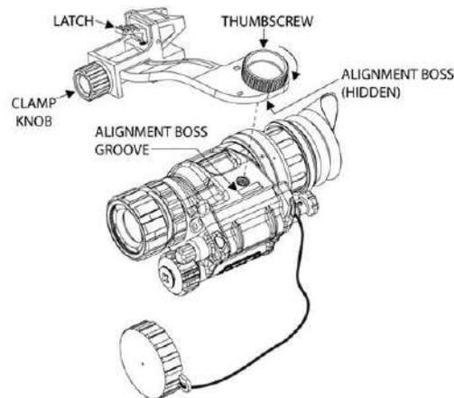
Figure 2-2 J-Arm Mount Adapter Installation
